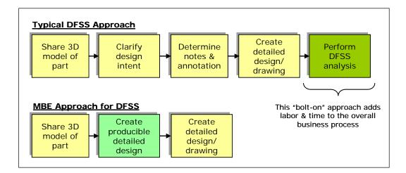
With MBE, the 3D CAD model should act as the centerpiece for technical collaboration. This enables informed consideration of cost and producibility in an integral way during the model's formative stage. This effectively eliminates the bolt-on approach, and as importantly transitions the role of manufacturing from being "design auditors" to actually helping to complete the detailed design.
